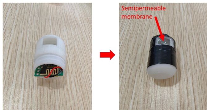
(a) The capsule robot prototype (b) After sealing Fig. 13 Before and after the capsule robot sealing
