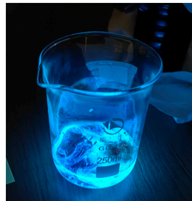
Fig. 12 The luminol chemiluminescence reaction
